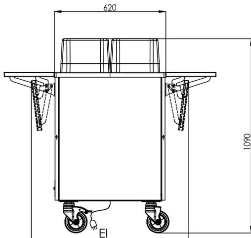
EI = Electrical inlet (power)  $\varnothing 80$
